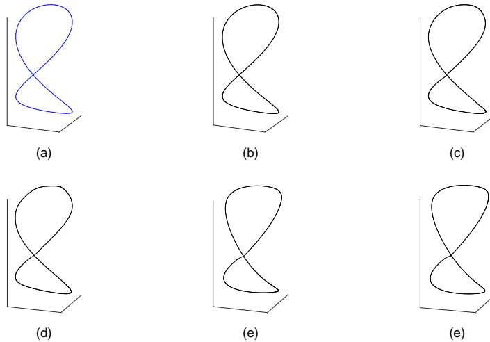
Figure 12 (a) the original curve, (b) result obtained with noise free data, (c)–(f) results obtained with noise intensity of 5%–20% in Example 4.4
